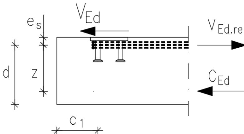
**Figure 6. Additional tensile force in additional reinforcement**
