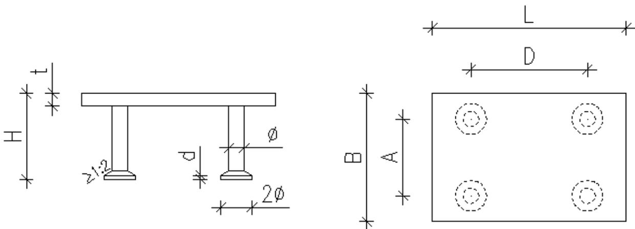
Figure 1. Dimension markings of SBKL fastening plates
